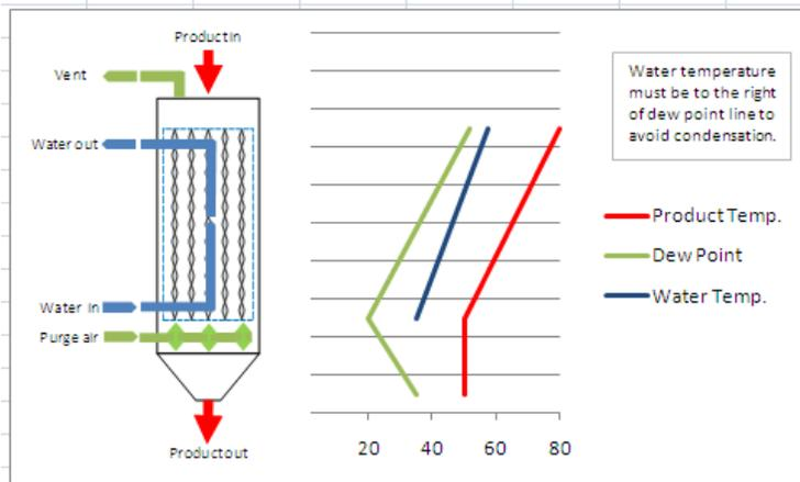
Figure 4 - Product Temperature and Dew Point through Heat Exchanger
