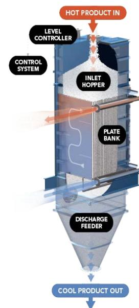
Figure 1 - 3D view of Bulk Solids Cooler
