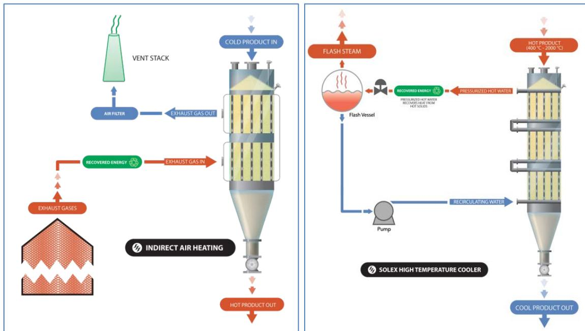
Figure 6 - Two examples of energy recovery, left - drying/heating of bulk product and right recovery of energy to generate pressurised water (for flash steam) through cooling of bulk product.
