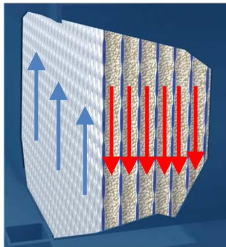
Figure 2 - Exchanger Plate with true counter-flow water
