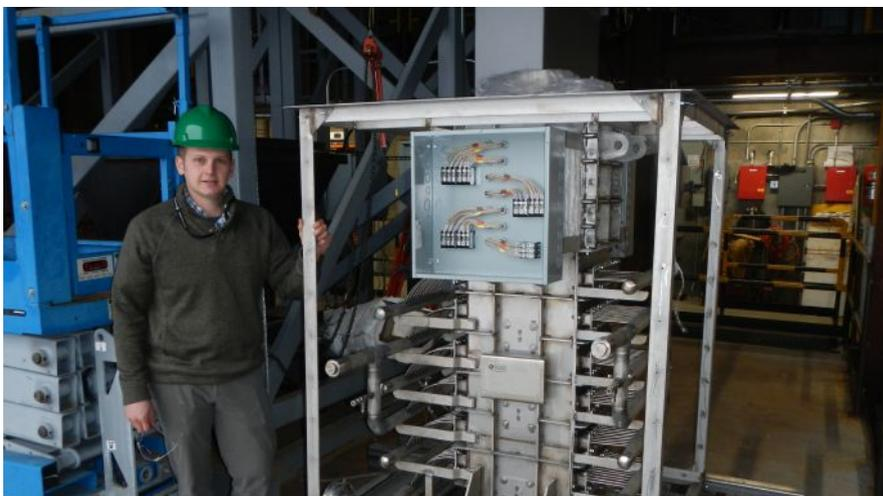
Kevin Albrecht, a mechanical engineer with Sandia National Laboratories, stands next to a particle-supercritical CO2 heat exchanger designed in collaboration with Solex Energy Science.
