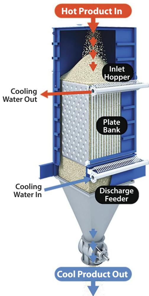
A bank of vertically arranged plates in the exchanger allows free-flowing bulk solids such as fertilizer, sugar and oilseeds to pass through while a separate stream such as water flows counter-currently within the plates. This allows for indirect heating, cooling or drying with the vertical plate heat exchanger. A discharge device at the bottom of the exchanger ensures uniform mass flow and consistent temperature profiles once material exits.
