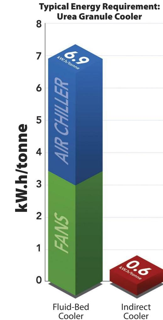
In urea granule applications, indirect heat exchangers consume up to 90 percent less energy than direct-contact alternatives such as fluid beds. (Energy consumption based on estimated operating power requirements, typical for a 3,600 tonnes per day urea plant in a U.S. Gulf Coast location.)
