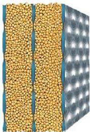
In a vertical bulk-solids heat exchanger, material passes between the plates through gravity while a fluid runs counter-currently within the plates. A discharge device at the bottom helps to ensure uniform mass flow and a consistent output temperature.
