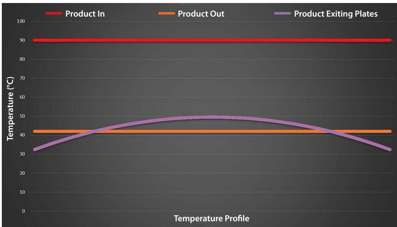
In this cooling application, a product at an average temperature of 194°F (90°C) is fed to an exchanger with a target average output of 107°F (42°C). The curved line shows the temperature profile between the plates, with the coldest product against the plates and the warmest in the middle. As the product travels vertically through the exchanger, the curved line begins to flatten out to the target output temperature.
