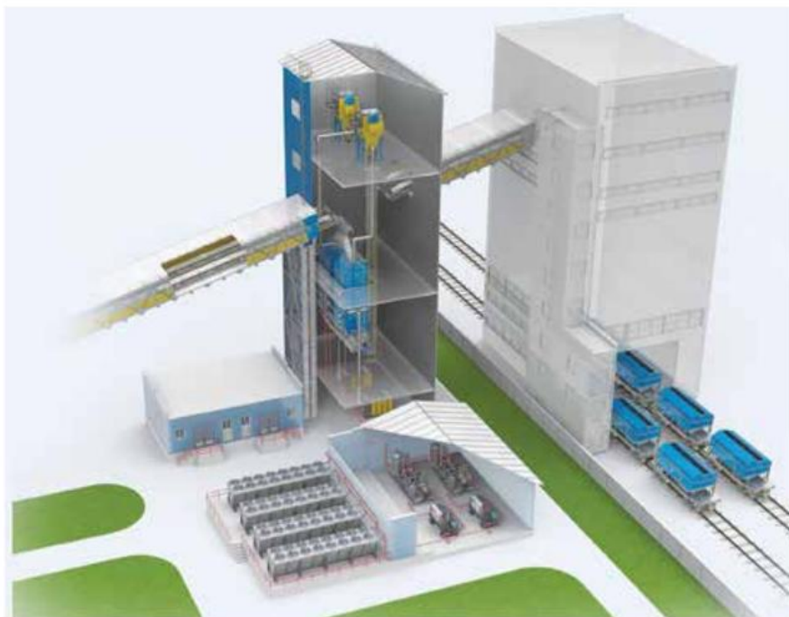
The vertical configuration of indirect heat exchangers means it can cool potash in pre-loading storage areas. PHOTO COURTESY OF SOLEX THERMAL SCIENCE.
