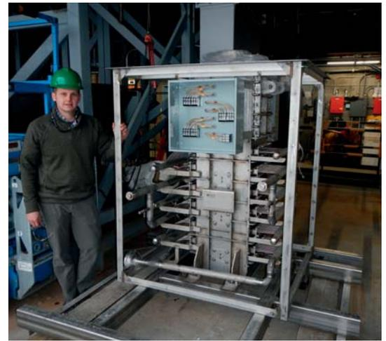
♣ A high-temperature heat exchanger with particulate solids and supercritical CO<sub>2</sub>, which part of a solar power research project carried out by Sandia National Laboratories in the U.S. Photo credit: Solex Energy Science
