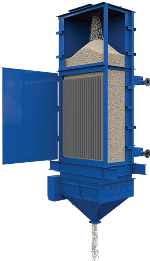
Indirect heat exchangers can consume up to 90% less energy than conventional technologies and in some cases allow for energy recovery loops, increasing overall efficiencies. Since the unit is fully enclosed, there are also no dust emissions. The modular design and small footprint allow for facility retrofits and simple capacity increases. With no moving parts and easy access to individual plates, maintenance costs are lowered, ensuring long term reliable operation.
