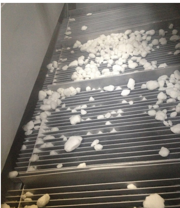
Figure 4. Obstructions at the top and/or within heat exchange plate banks can occur when off-spec particle size materials are introduced.
