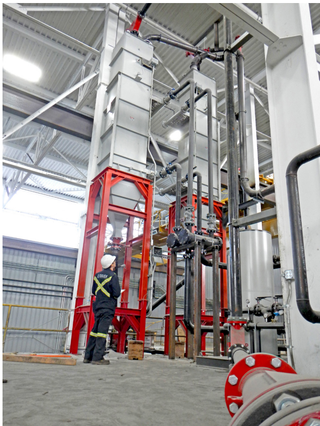
Figure 1. Moving bed heat exchangers (MBHEs) combine the thermal efficiency of plate heat exchange design with the science of uniform mass flow to cool a full range of urea, nitrate- and phosphate-based products.
