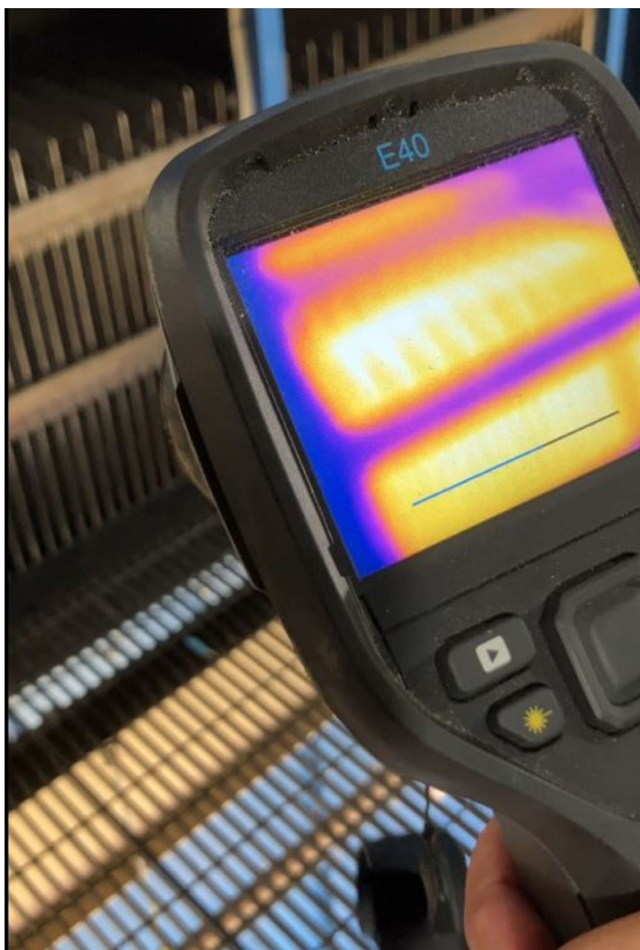
Figure 6. A heat camera can be used to diagnose whether specific spots of the heat exchanger plates are heating up more than others, or indicate if there is poor flow of the heat transfer fluid within the plates.
