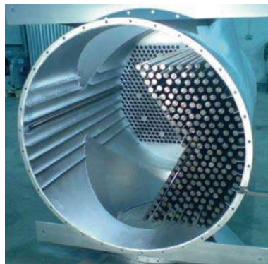
Econotherm's heat pipe heat exchanger equipment incorporates patented superconductor technology –and is highly efficient at recovering waste heat from process exhaust gases.
