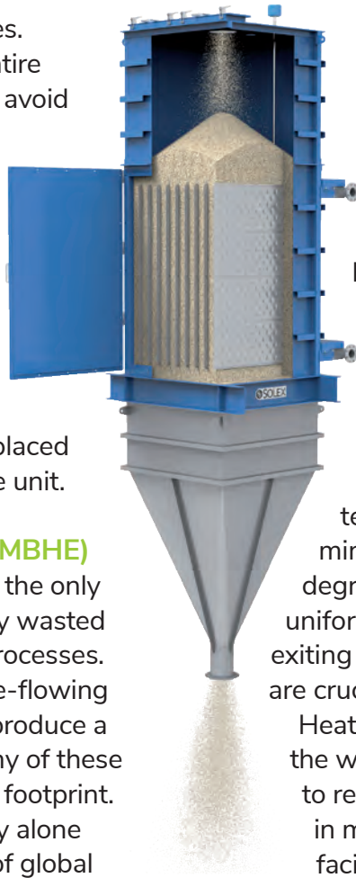
Figure 3 A plate-based MBHE illustrating how the product enters the unit from the top and flows by gravity through vertically orientated banks of stainless steel pillow plates (Source: Solex Thermal Science)
