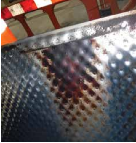
⚠ Foreign material that enters the heat exchanger can cause blockages (e.g. plugging), leading to high velocity flow zones that are manifested by areas of discoloration on the plates.
