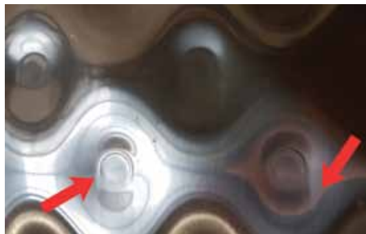
➤ This plate shows examples of where the laser weld is both fading (left) as well as striations are showing (right).
