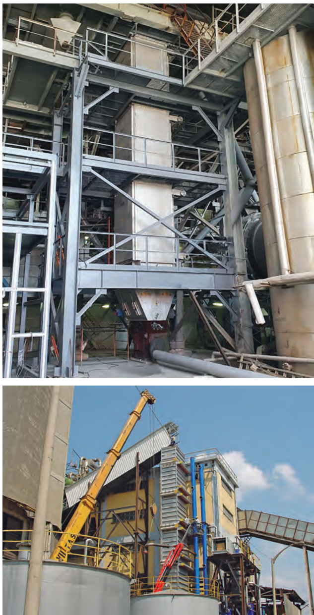
Figure 3. For decades, MBHEs based on vertical plate technology have acted as cornerstones in the fertilizer production process (Source: Solex Thermal Science).
