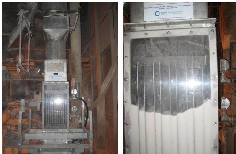
**Fig. 2.** Pilot unit used for the testing amorphous sugar with Plexiglas window to allow observation of flow.
