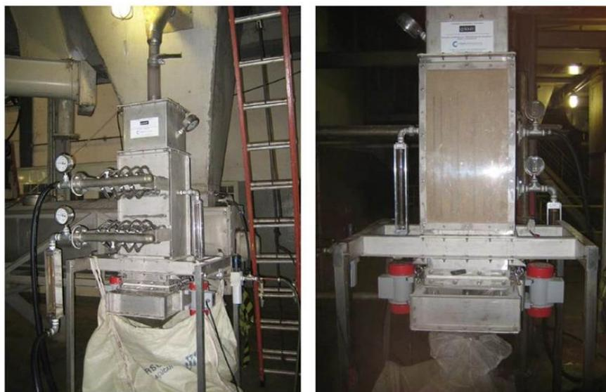
**Fig. 3.** Pilot unit fitted with a Plexiglas front used to test raw sugar.
